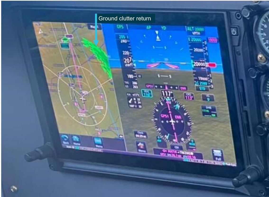
Figure 8: Weather radar ground clutter on VH-ZMW
