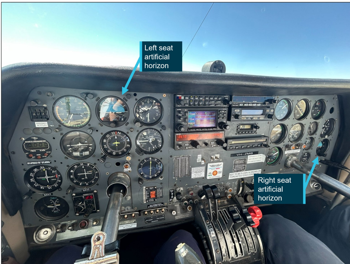
Figure 2: Photo of cockpit instruments from perspective of left (pilot) seat
