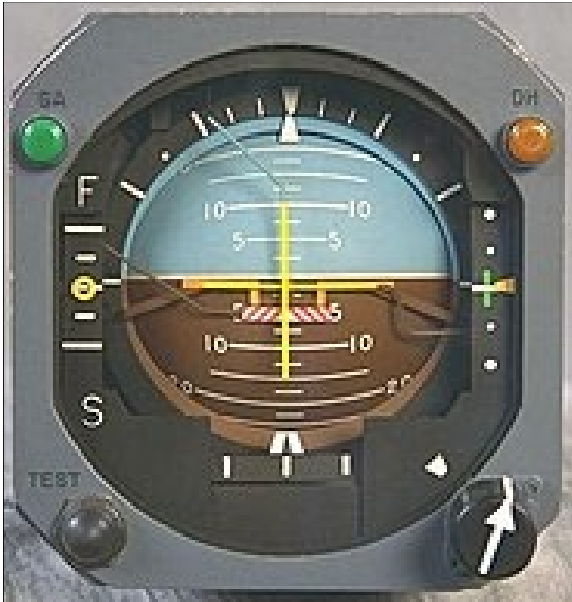
Figure 5: Generic example of an artificial horizon
