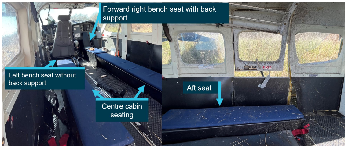
Figure 6: VH-UMV cabin seating arrangement
