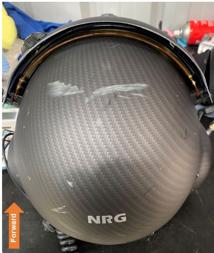
Figure 7: Top view of helmet worn by the pilot of VH-ZDI showing damage
