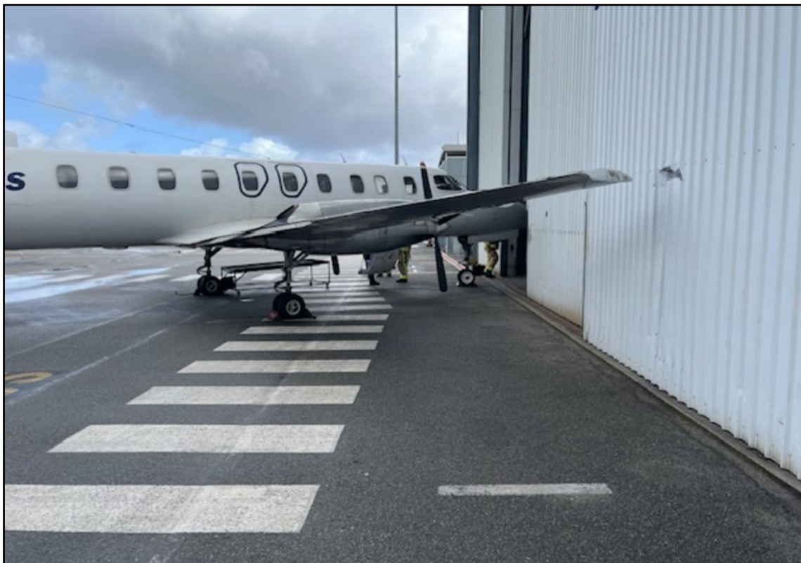
Figure 2: VH-WAJ shown stationary after collision with operator’s hangar
