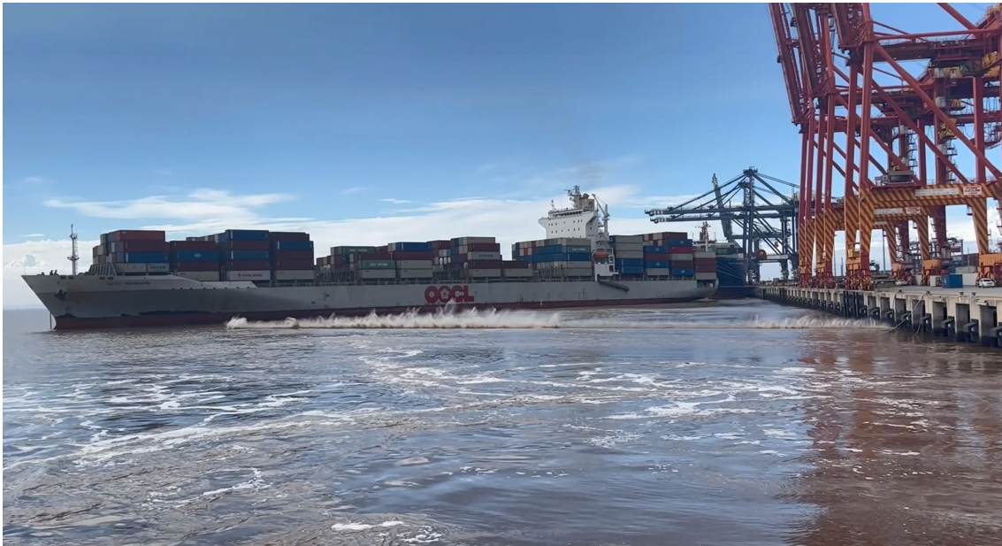
Figure 5: OOCL Brisbane breaking away (image shows the last headline parting)
