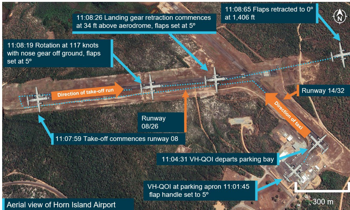
Figure 1: QAR derived flight data depicting aircraft position and flap setting
