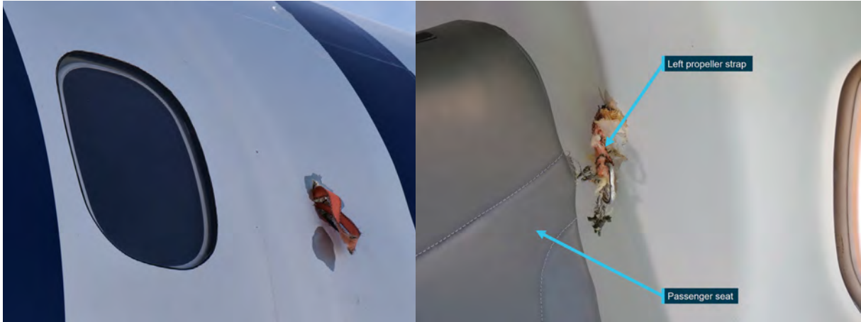
Part of the left propeller strap that entered the fuselage adjacent to seat 2A
