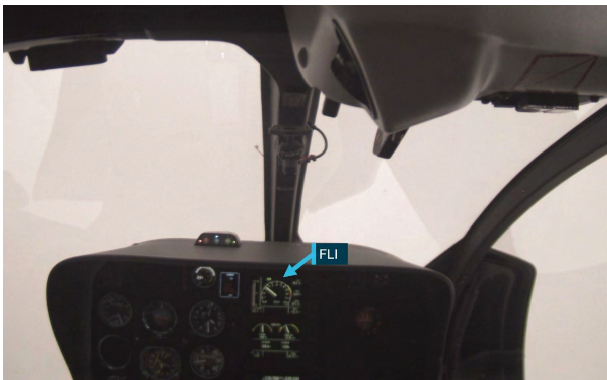
On board footage of weather conditions from the accident helicopter, 22 seconds before the collision with terrain
