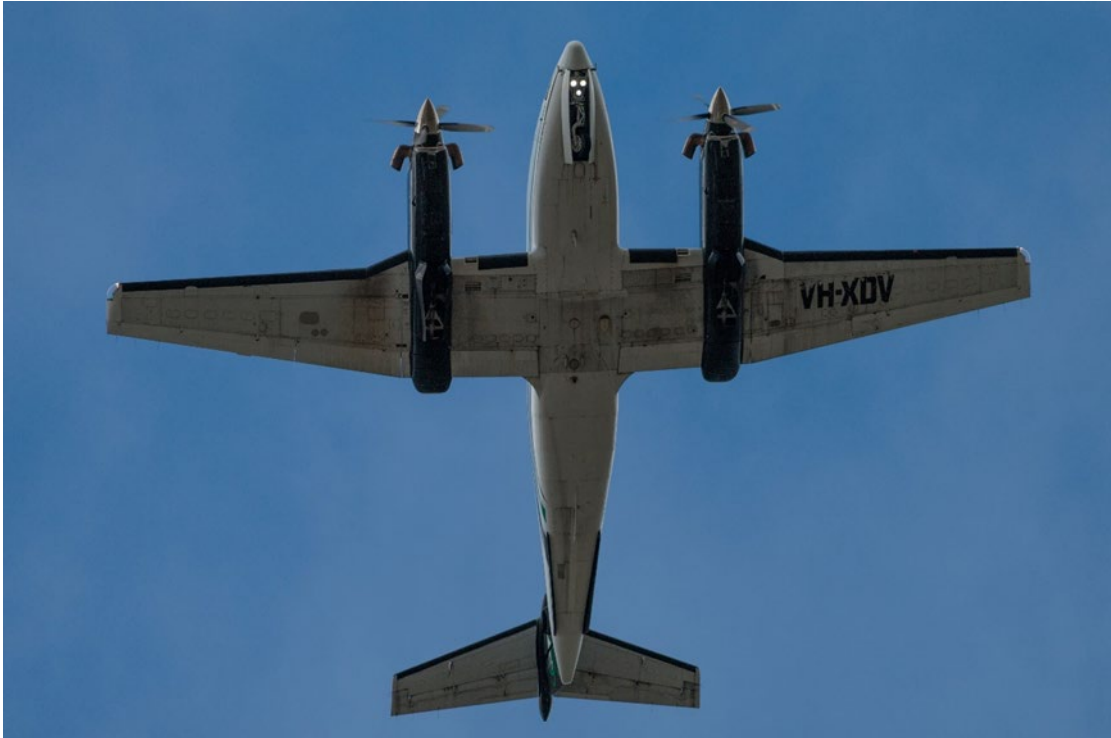
Figure 1: VH-XDV with landing gear partially retracted as it overflew Williamtown Airport
