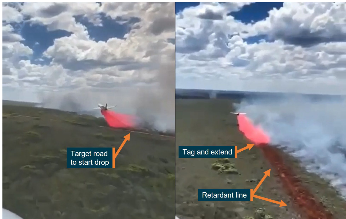
Figure 12: First drop (left) starting at road and second drop (right) tag and extend
