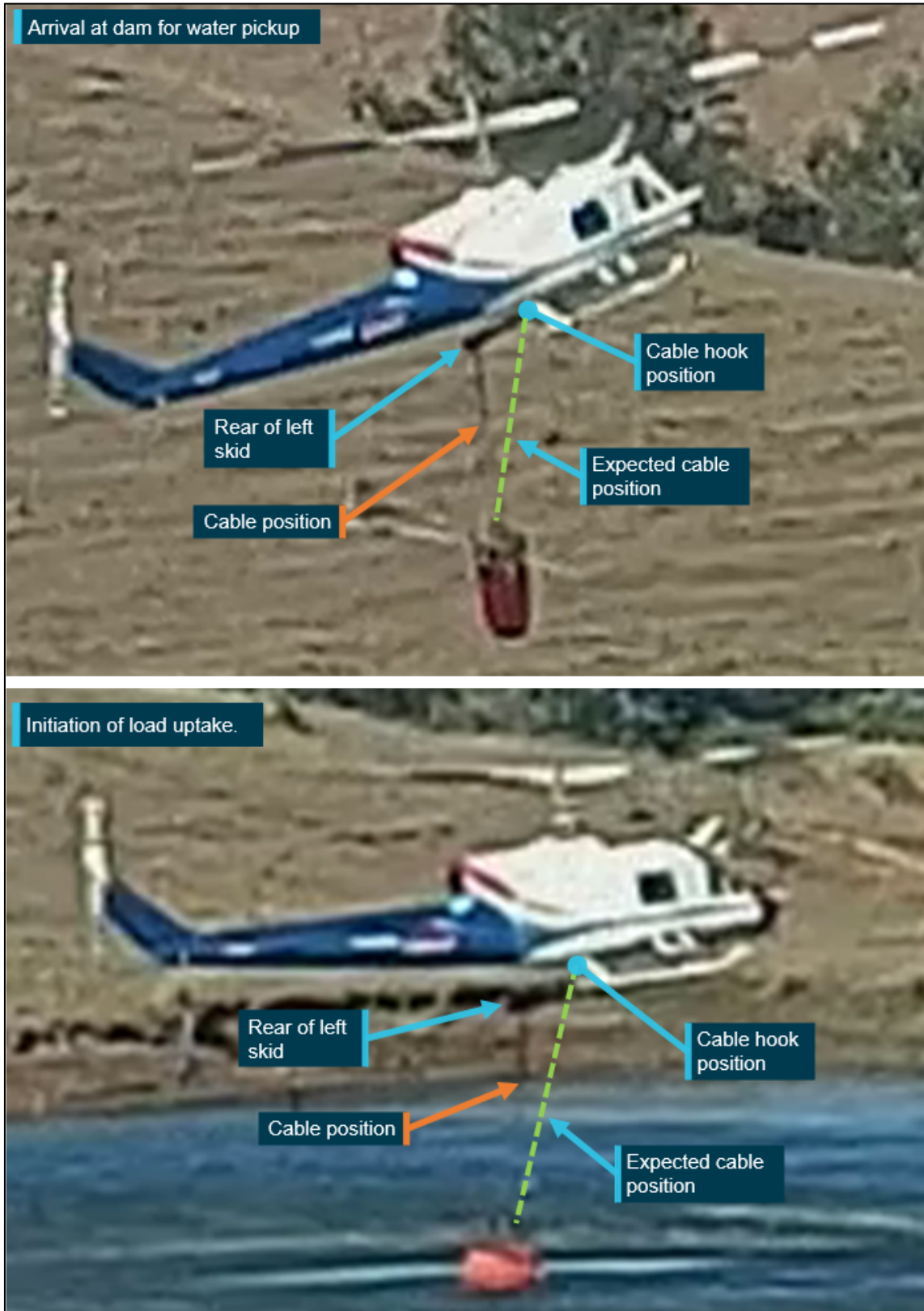
Figure 3: Sequence of water pickup from dam showing bucket cable position from approach (top) to lifting off (lower)
