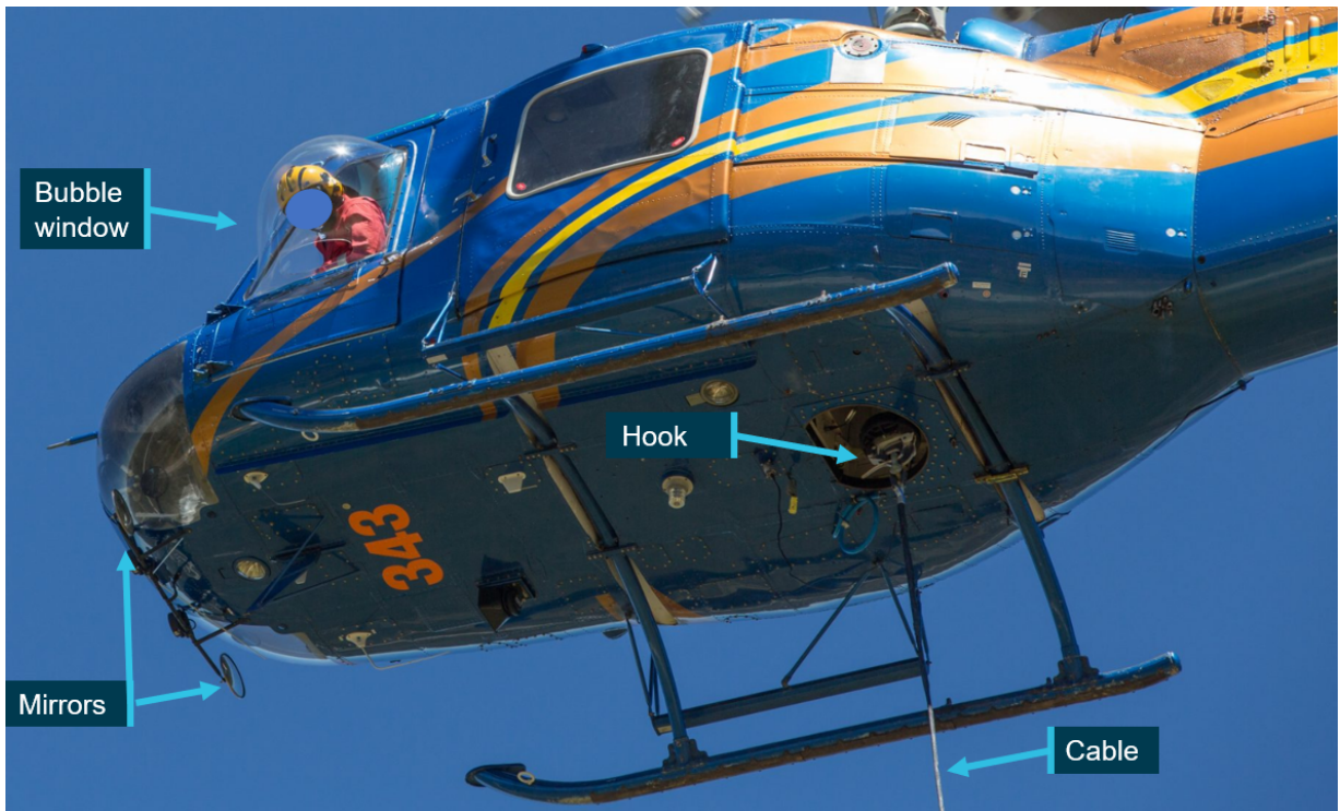
Figure 5: Bell 204 showing mirrors and bubble window
