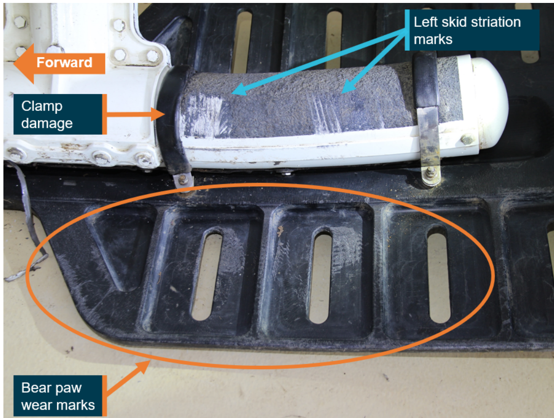
Figure 8: Left rear skid showing corresponding skid and bear paw damage
