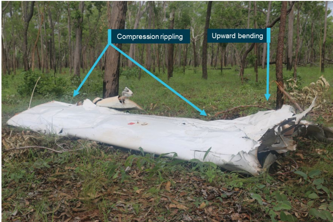
Figure 10: The right wing showed compression rippling of the upper skin surface and permanent deformation from exposure to upward bending
