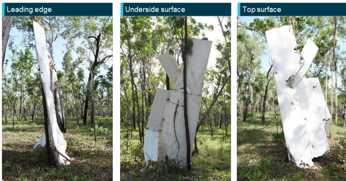
Figure 9: The right wing as it was found approximately 300 m from the main wreckage
