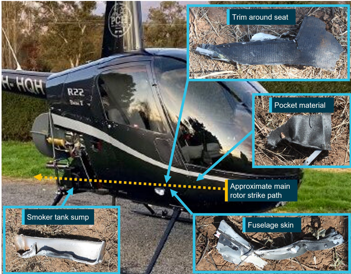
Figure 4: VH-HQH (pre-accident) showing approximate location of rotor strike location and locations of first items in debris field
