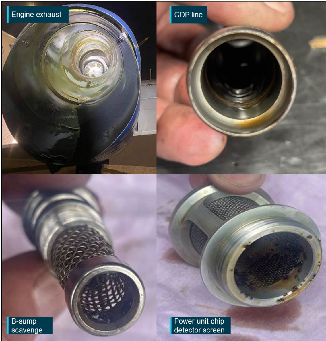
Oil located in engine exhaust and CDP line. Debris located in B-sump scavenge and power unit chip detector screens Source: Regional Express, annotated by the ATSB
