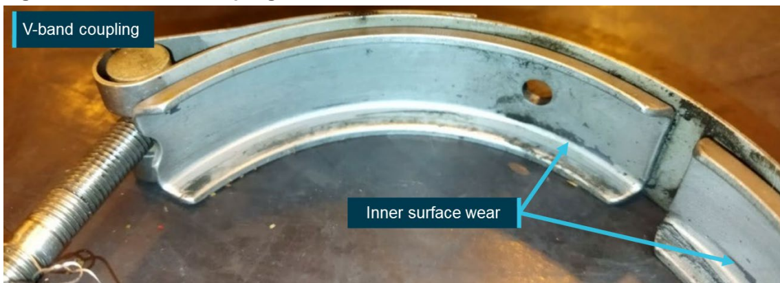
Figure 7: HMU V-band coupling wear location
