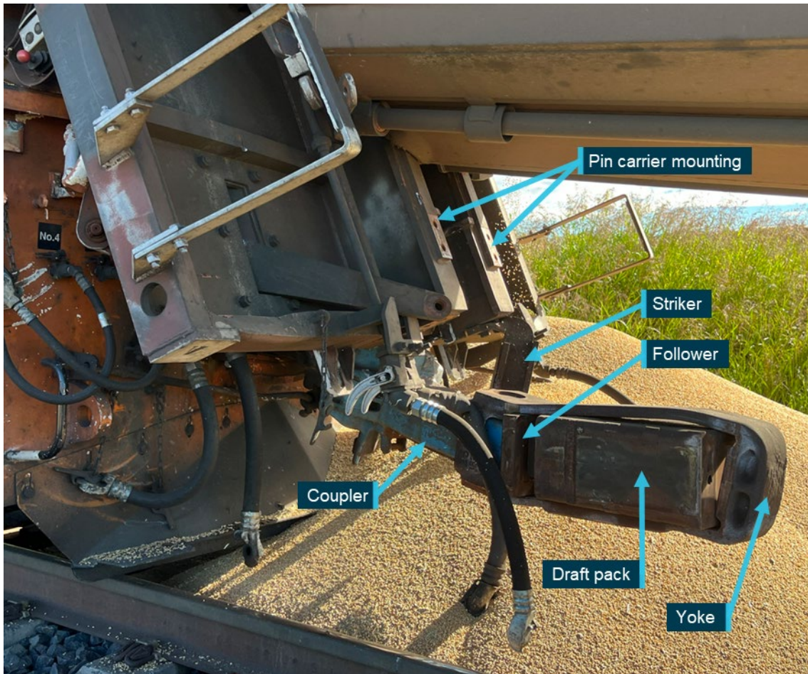
Figure 16: Wagon BGKF 1122F coupler components
