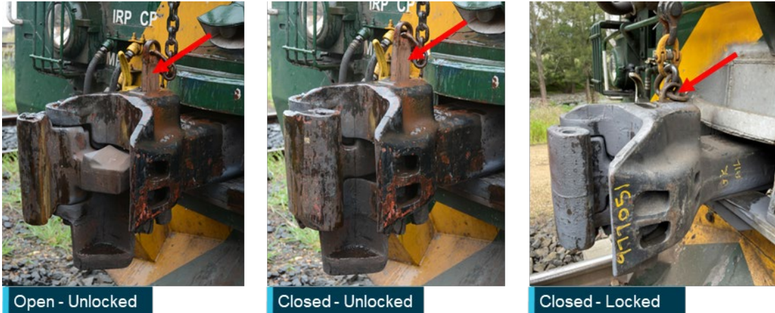
Visual appearance of the lifter in various operational knuckle states for a top lifter operated automatic coupler. Source: OTSI
