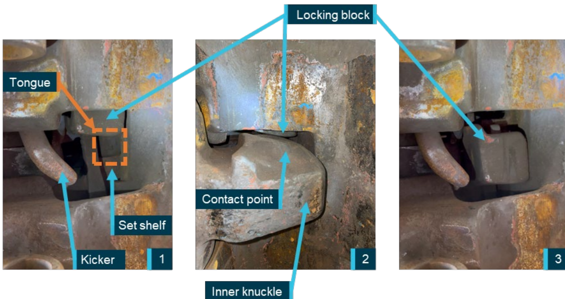
Figure 11: Internal coupler mechanisms
