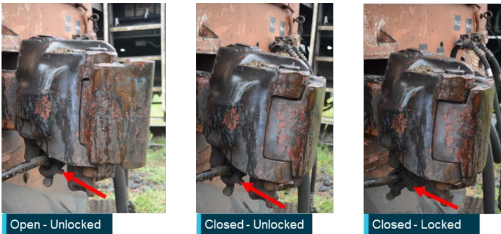
Visual appearance of the lifter in various operational knuckle states for the bottom lifter operated automatic coupler that was fitted to locomotive L277, the accident locomotive. Note: the coupler has been bent downwards from the accident. Source: OTSI
