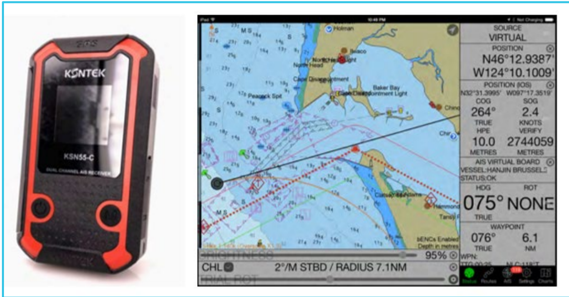
Figure 14: KSN55-C model PPU and example SEAiQ chart display on a tablet device
