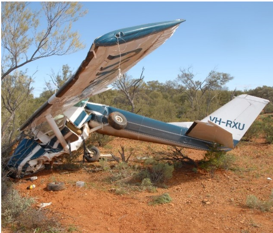
Figure 2: Photograph showing the accident site terrain and impact damage to the aircraft.
