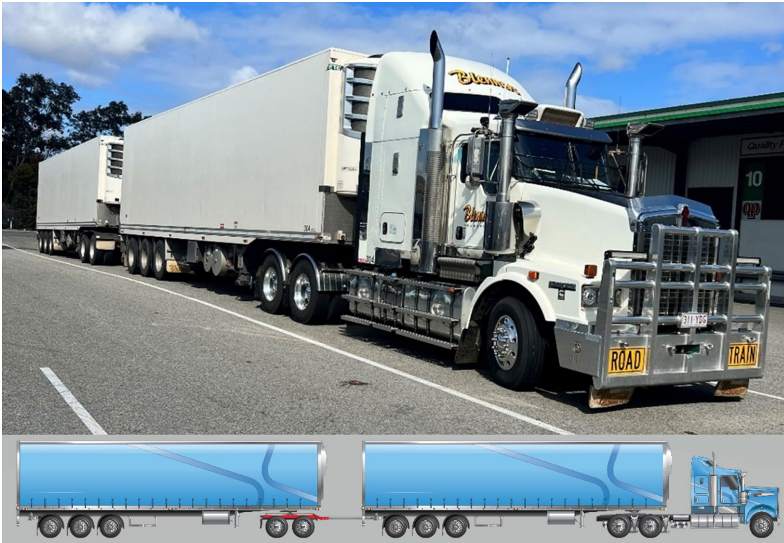
Figure 3: Truck configuration prior to collision
