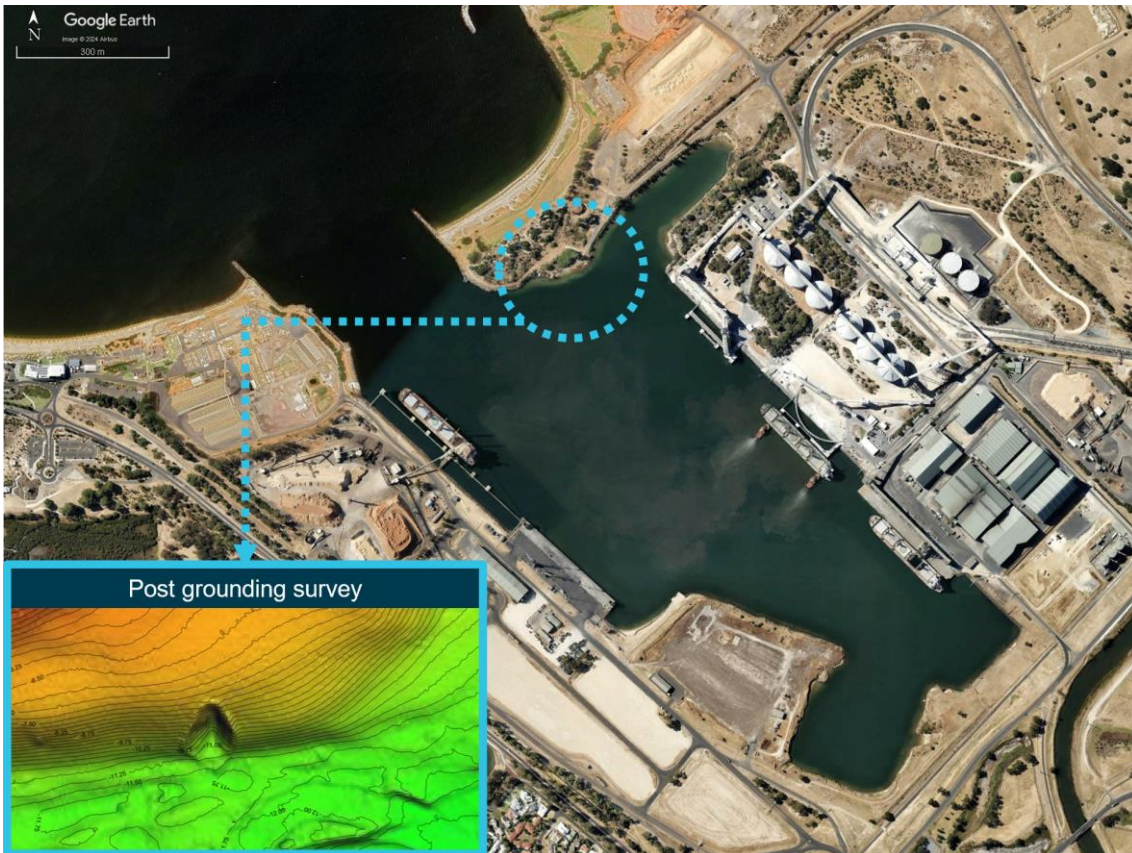
Figure 2: Post incident survey imagery of shallow water (circled)
