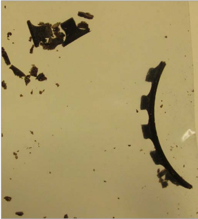
Figure 2: Pieces of the failed phenolic bearing cage
