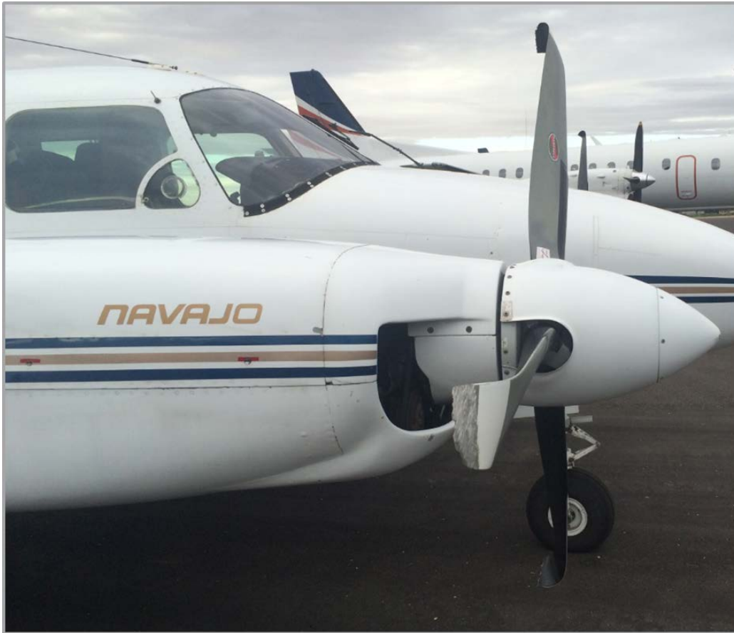
Figure 3: Damage to ETW propellers
