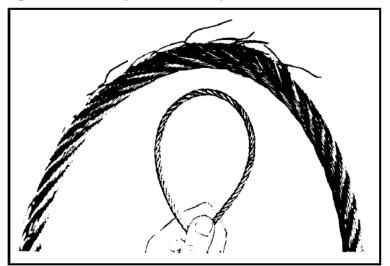
Figure 5: Cable inspection technique
