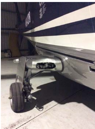
Figure 2: Damage to right landing light of VH-XPB
