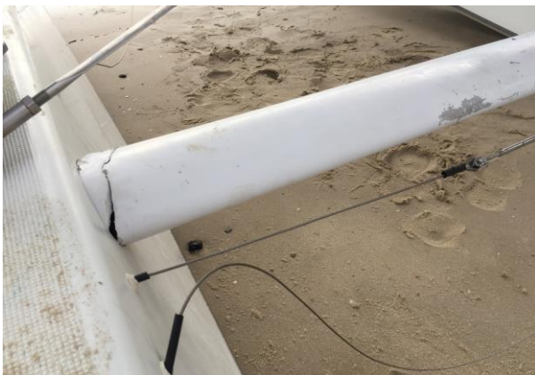
Figure 3: VH-NTK rear strut fracture (view of the left float facing forwards)
