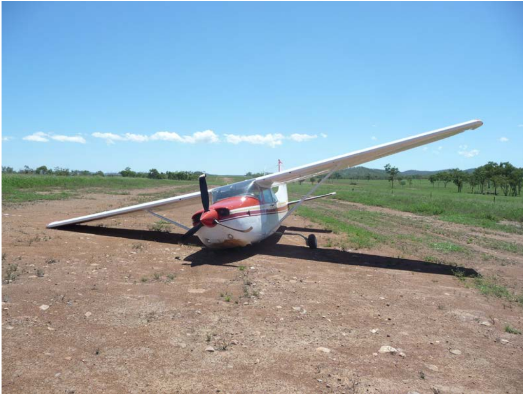
Figure 2: VH-PFZ showing retracted nose wheel and right landing gear, and damaged propeller
