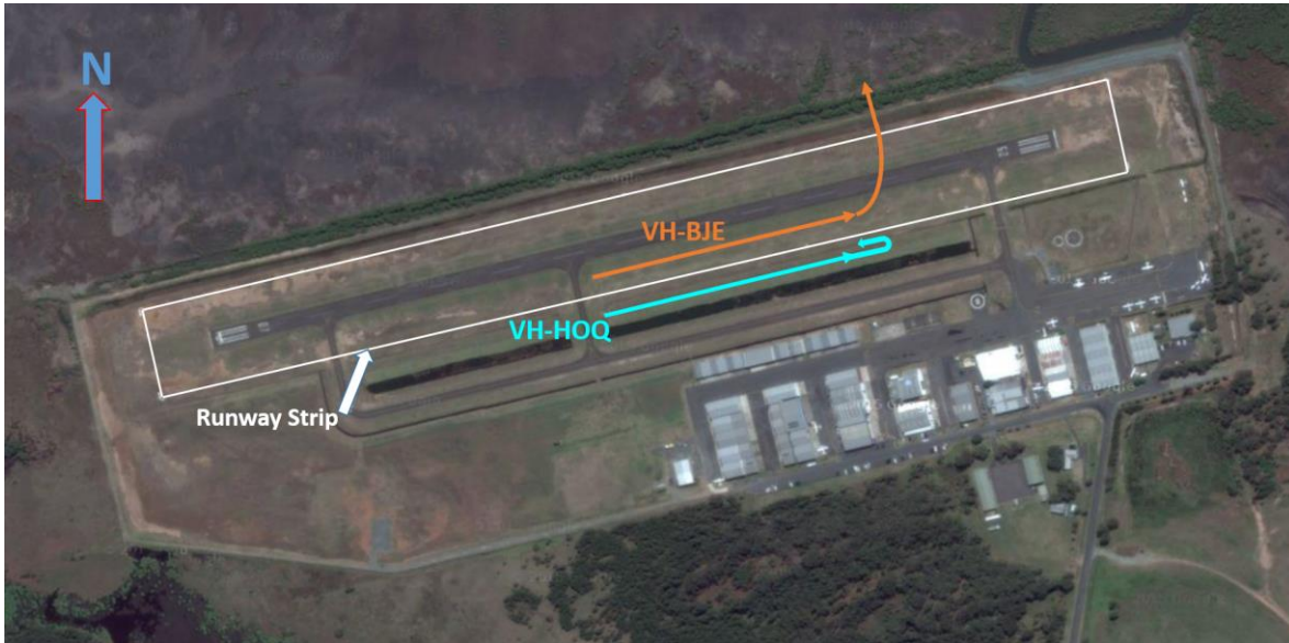
Figure 3: Redcliffe aerodrome showing the runway strip (white). The take-off run and left turn of BJE is indicated in orange. The track of HOQ when conducting the engine failures during taxi and the reversal turn is indicated in blue.
