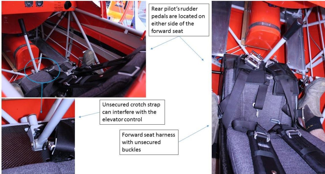
Figure A3: Possible elevator control interference from an unsecured forward seat harness
