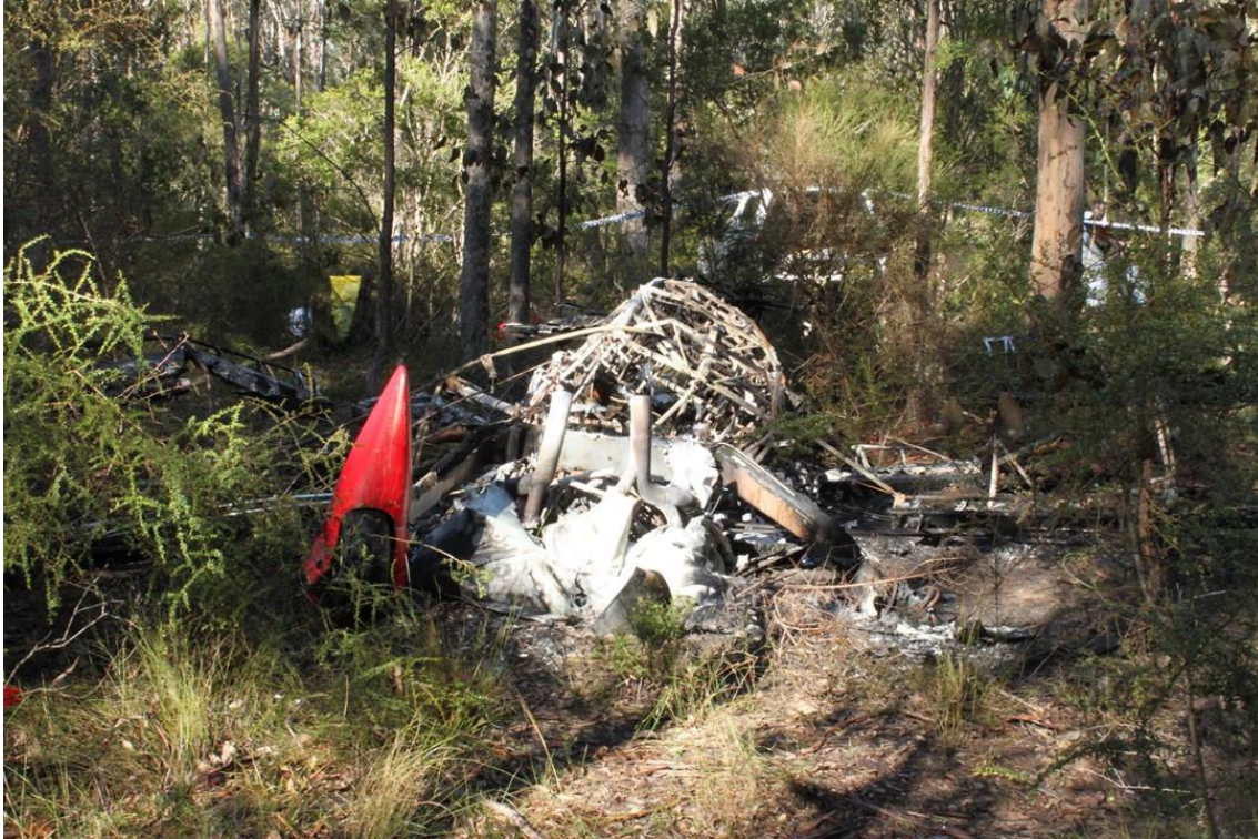
Figure 1: Accident site viewed from the front of the aircraft and showing the surrounding thick vegetation and minimal structural damage to the wings and airframe (consistent with the reported vertical descent)
