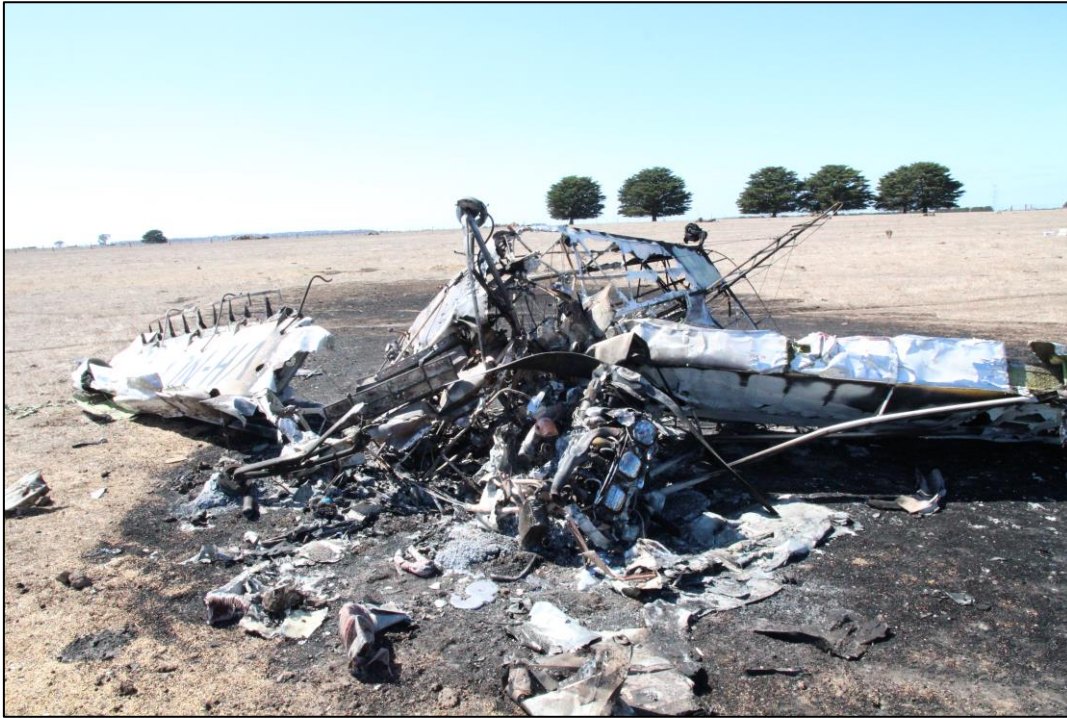
Figure 1: Aircraft wreckage (looking east), showing the lower surface of the aeroplane. Note the significant damage to the forward fuselage and cockpit area and the extent of the fire damage to the fuselage and inboard wing sections
