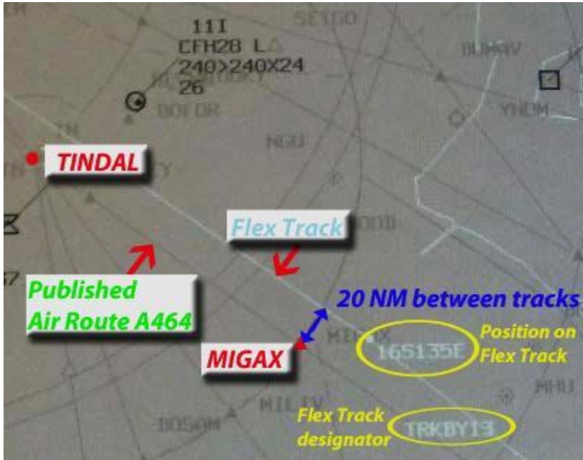
Figure 6: Air situation display image of track positions at the time of the occurrence showing flex track labels and involved tracks and routes
