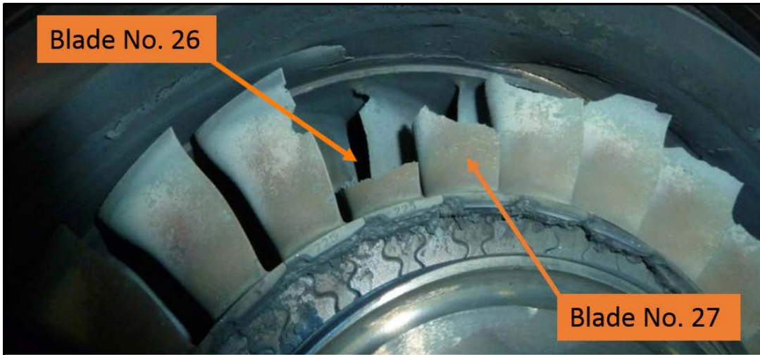
Figure 5: Blade No. 26 and damage to the adjacent blades
