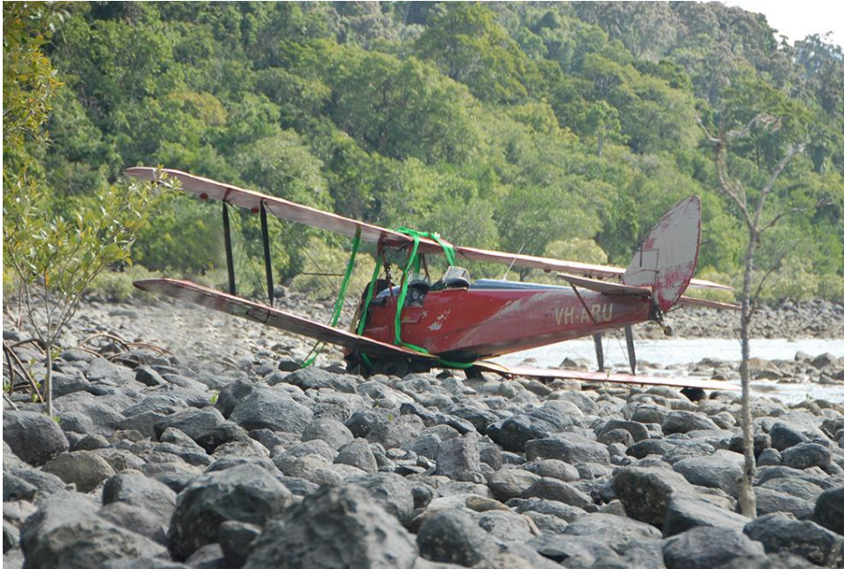
Figure 2: Accident site showing damage to VH-ARU
