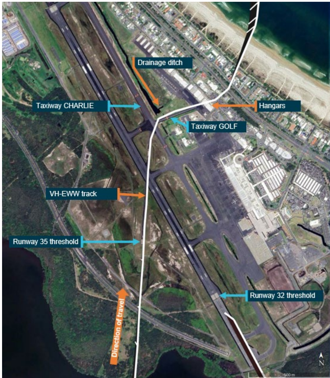
Figure 4: Gold Coast Airport taxiways CHARLIE and GOLF, drainage ditch, hangars and VH-EWW track
