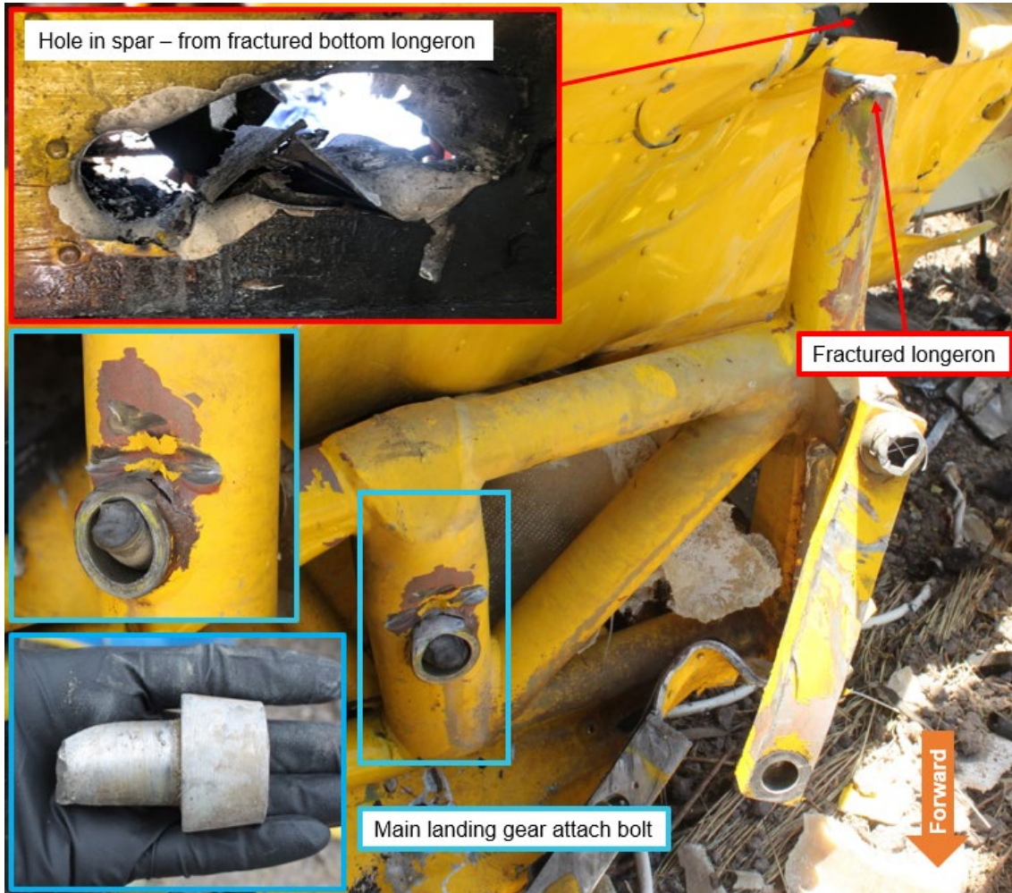
Figure 11: Fuselage frame longeron fracture and associated impact damage with main spar damage to right wing
