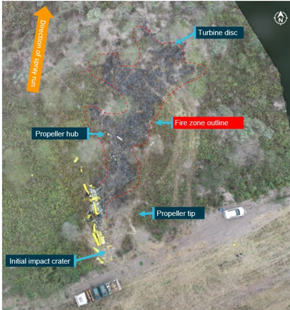
Figure 12: Overview of accident site and fire zone
