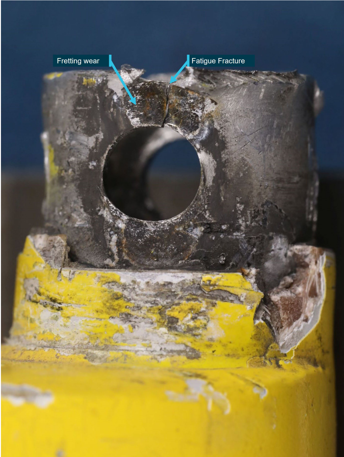
Figure 7: Rudder sleeve wear from contact with washer, and associated cracking
