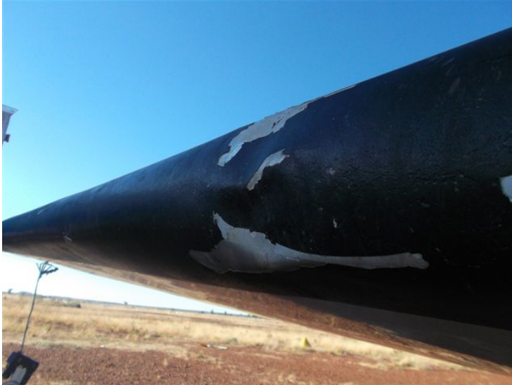
Figure 2: Damage to leading edge
