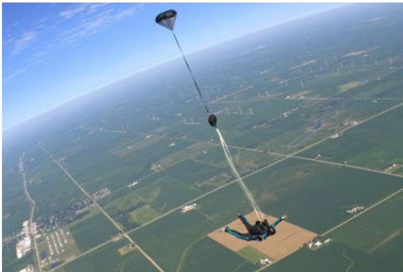
Normal deployment: Throw-away pilot chute connected to main deployment-bag, just prior to bag opening.
