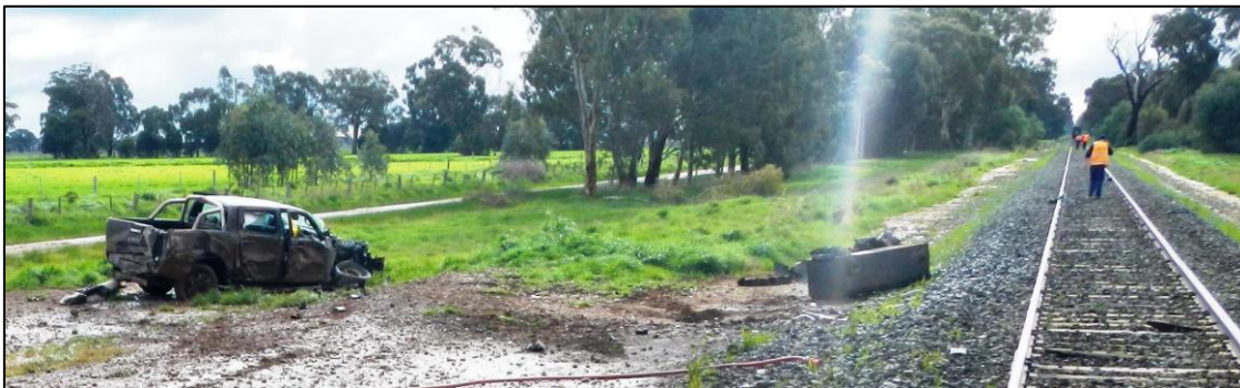
Figure 3: Damaged road vehicle and the fuel tank from the impacted rail car.
