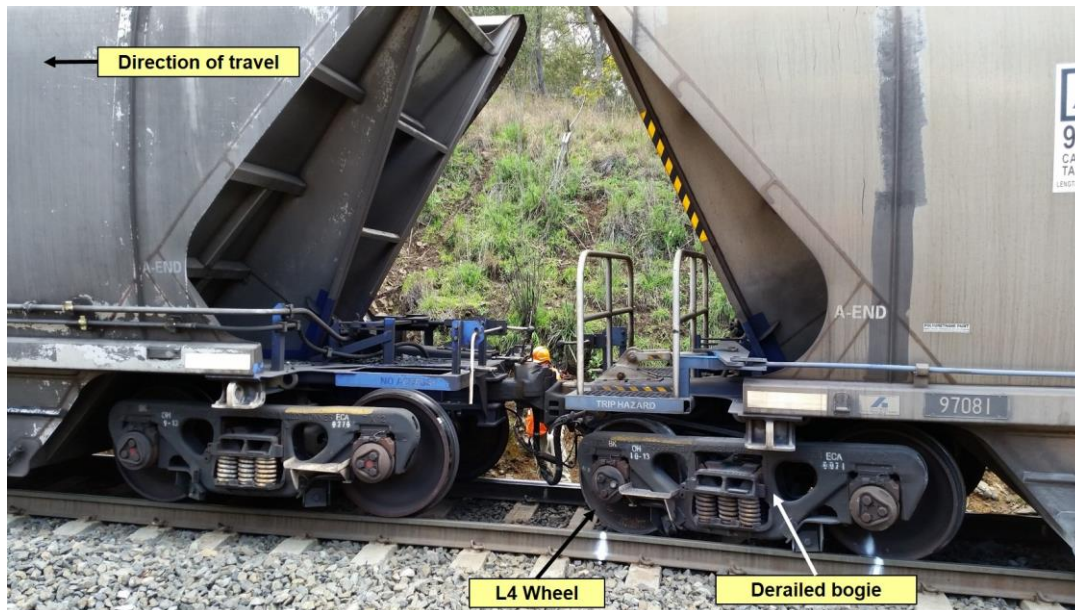
Figure 5: Derailed bogie viewed from Up side of track
