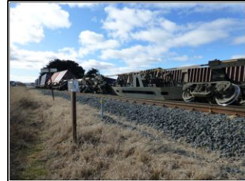
Derailed portion of train 532
