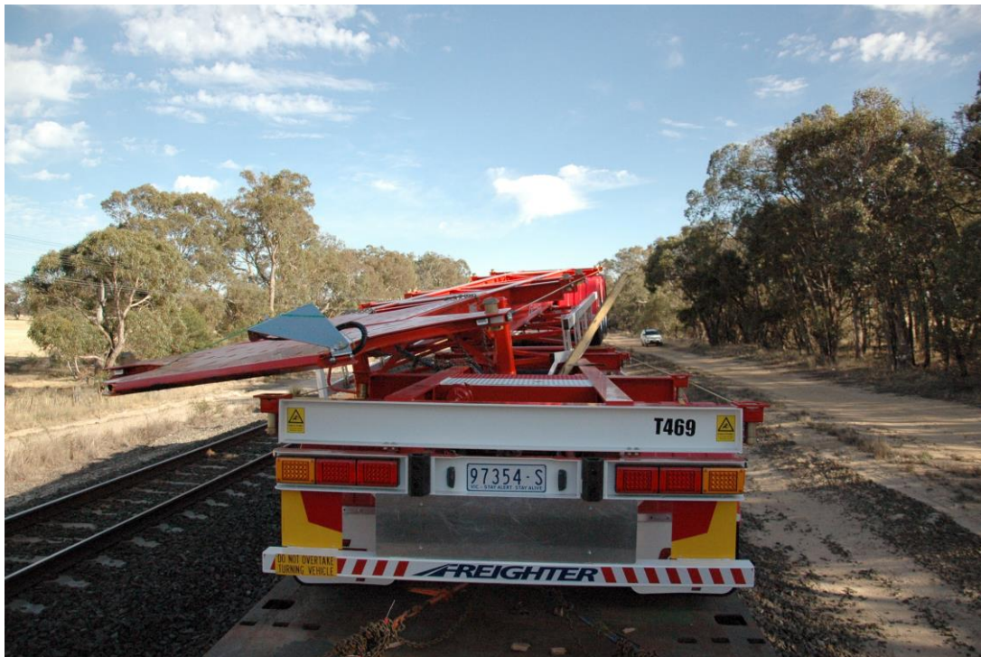
The top road trailer had shifted to the left-hand-side in direction of travel. The movement was enough to strike the bridge infrastructure. Source: SCT Logistics
