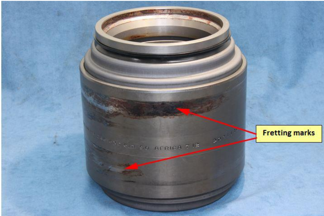
The corresponding fretting marks found on the partner-bearing cup was also evident on the partner swing arm. Source: ATSB
