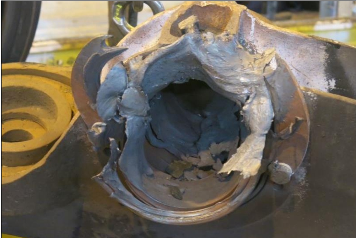
The XPT bogie swing-arm bearing housing, viewed from the inboard side. The heat damage is evident and the remaining bearing components can be seen inside the housing. Source: ATSB
