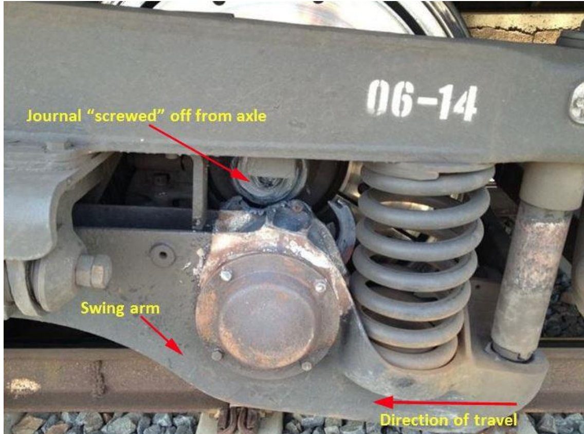
Figure 2: Failed axle and swing arm hanging down.
