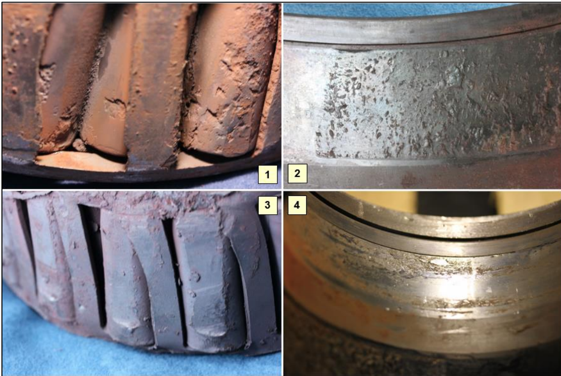
The remains of the failed bearing, obtained from within the swing-arm bearing housing. Image 1: Inboard cone, showing flattened, misaligned rollers with spalling fatigued surfaces. Image 2: Inboard raceway, showing full-width spalling fatigue. Image 3: Outboard cone, showing flattened rollers. Image 4: Outboard raceway showing full-width galling and deposited metal. Source: ATSB
