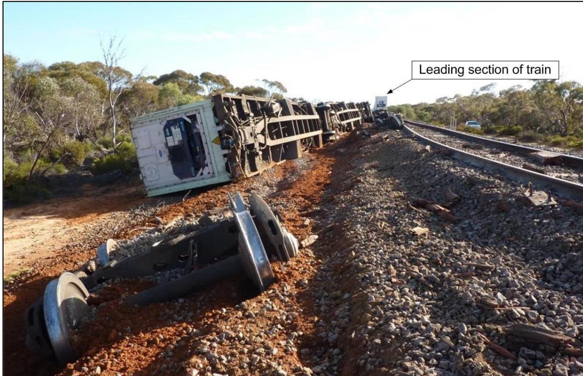
Figure 3: Leading section on rails and rolled wagons
