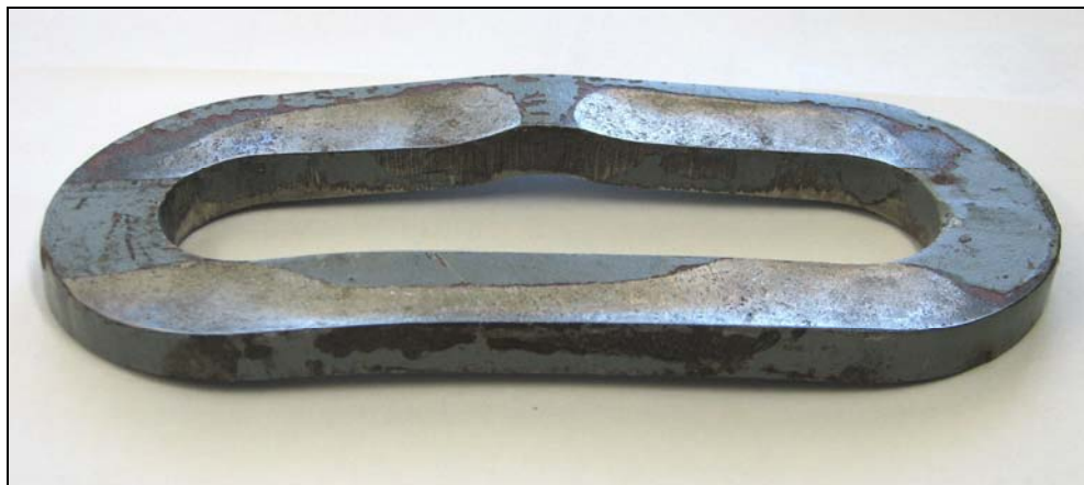
Figure 10: Draft key anti-wear collar from CQBY 0118A showing wear and deformation
