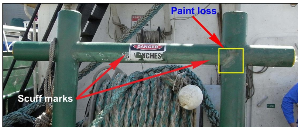
Figure 21: Heeling of Adonis , indicating the towline position in the 'H' bitts
