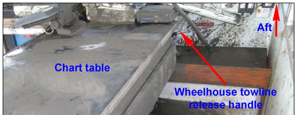
Figure 23: Position of the wheelhouse towline release handle
