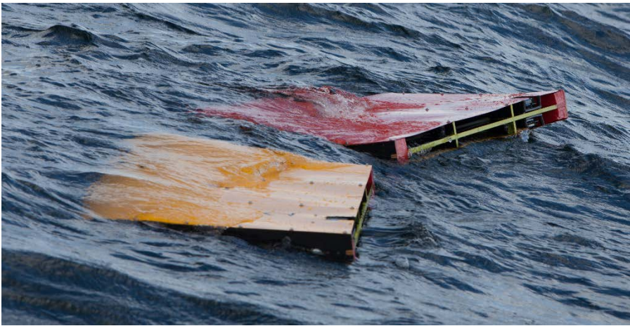
Figure 2.3.1 Replica flaperons at sea off Maria Island, Tasmania, one deployed with the extrados (orange surface) up and one with the intrados (red) up. Both self-oriented with the raised trailing edge to windward. GPS units can be seen in their cut-outs.
