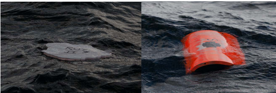
Figure 2.3.3 Replicas of 'Roy' (first seen at Mossel Bay, South Africa on 23 Dec 2015) and the piece of flap track fairing (found on Daghatane Beach, Mozambique, on 27 Dec 2015). GPS units are embedded.
