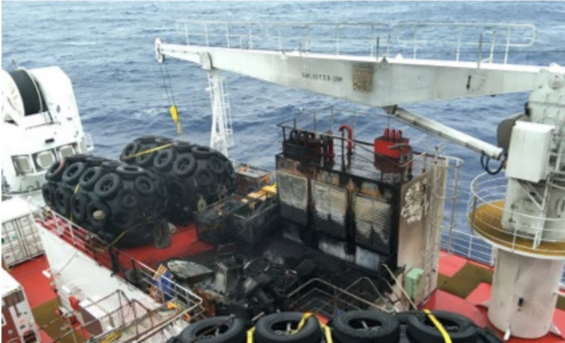
Figure 5: Fire damage on deck including the burnt-out watercraft adjacent to the casing
