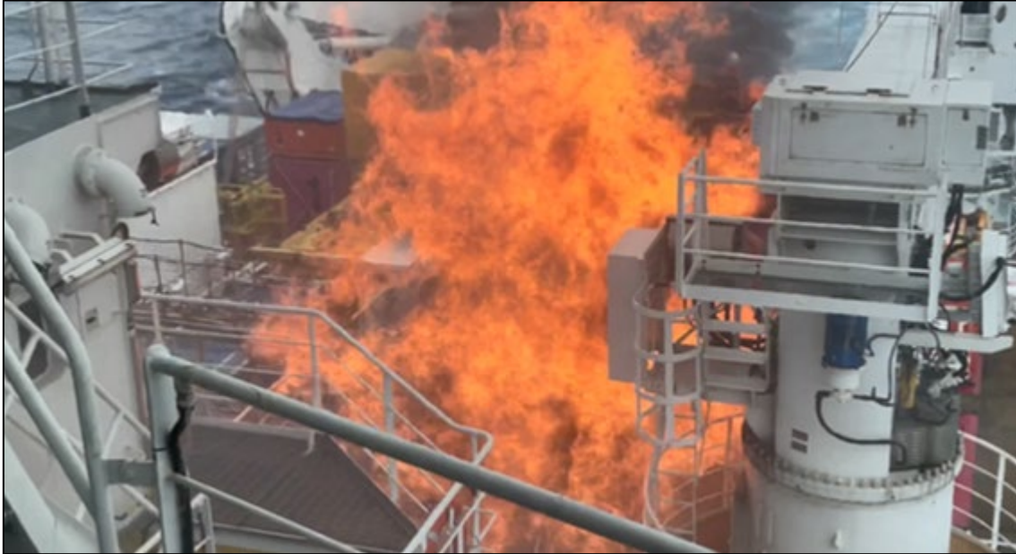
Figure 4: Flames from the port engine room exhaust casing
