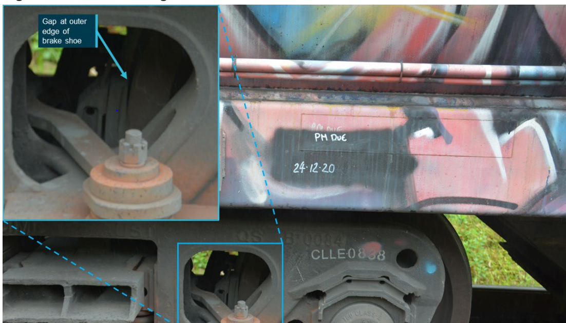
Figure 18: Side of 1 st wagon CGSY 04516T brake shoe
