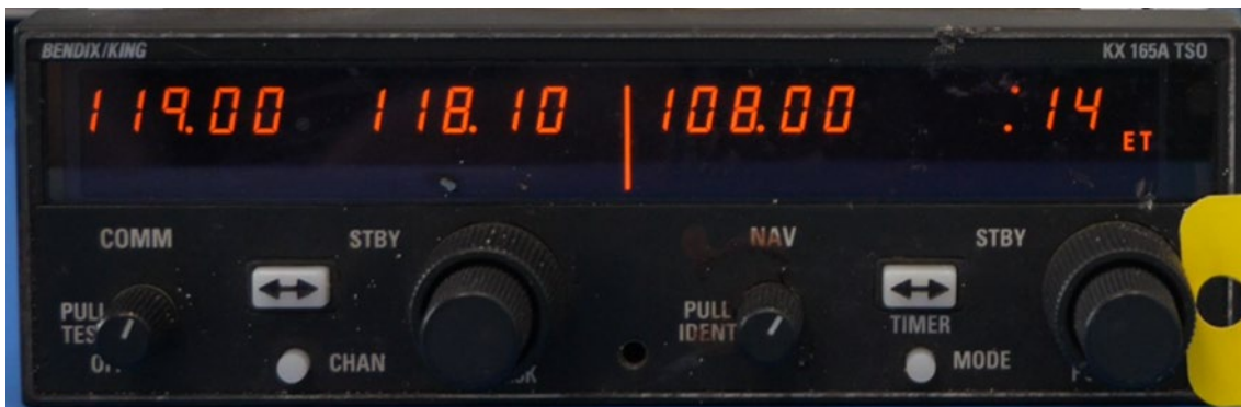
Figure 5: Bendix King KX-165A from VH-XH9 - Indication on power up
