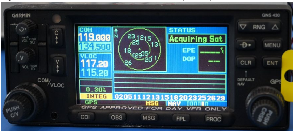
Figure 8: Garmin GNS430 from VH-XKQ - Indication on power up after self-test
