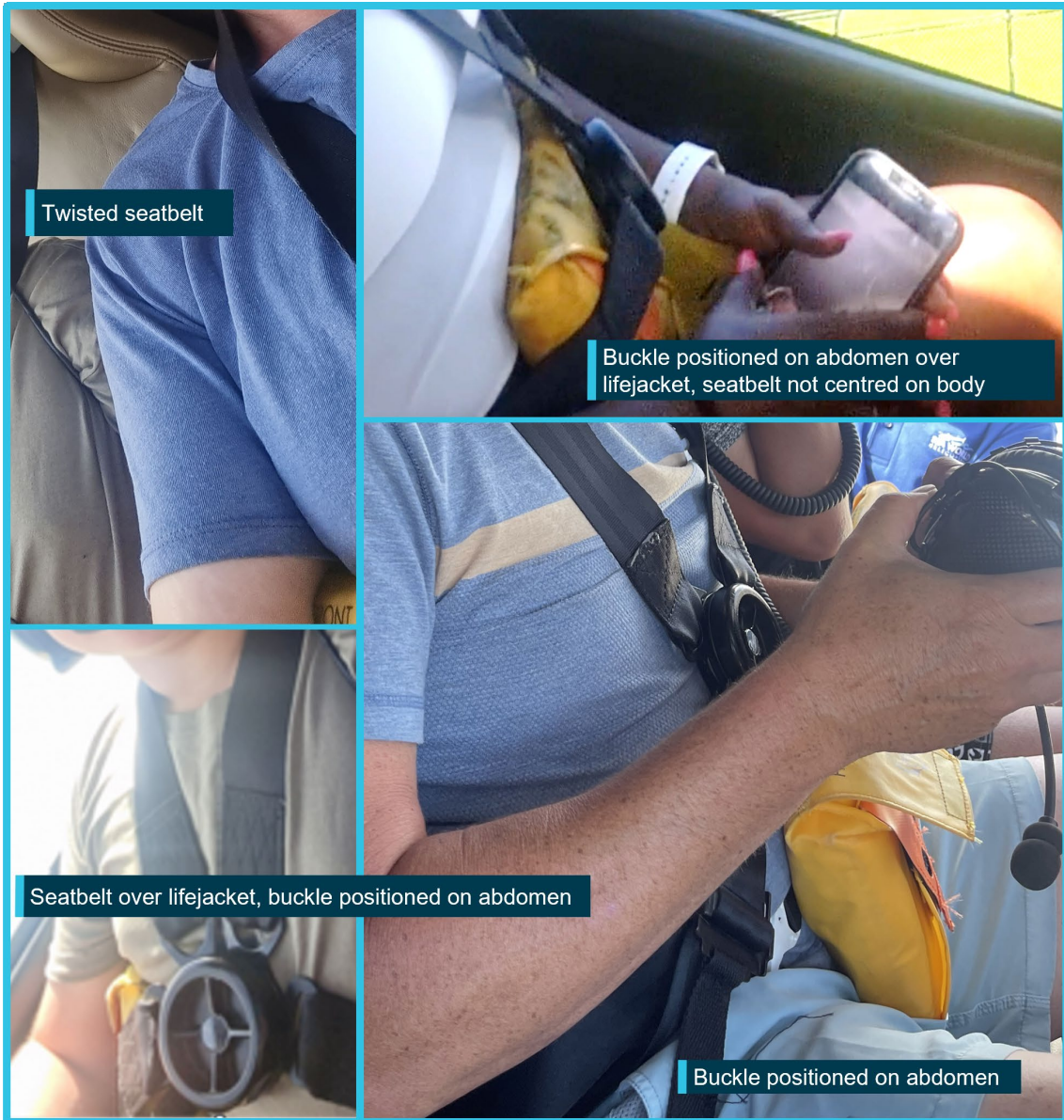
Figure 20: Examples of passenger incorrect seatbelt fitment
