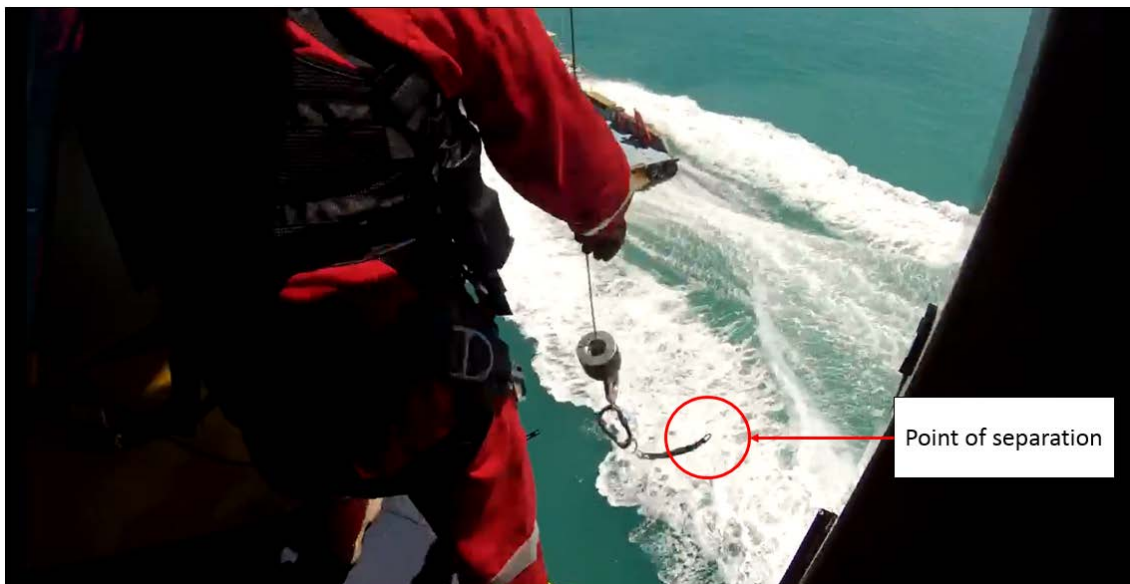
Figure 2: Weak-link point of separation
