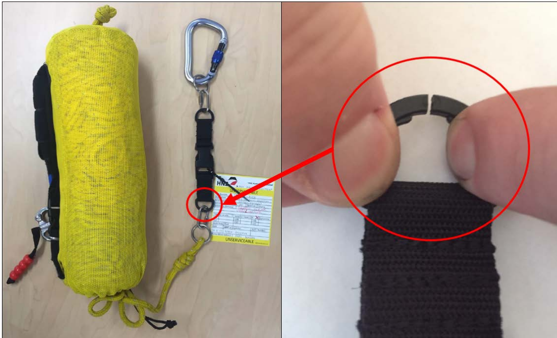
Figure 3: Hi-line with weak-link and carabiner (left) and fractured weak-link (right)
