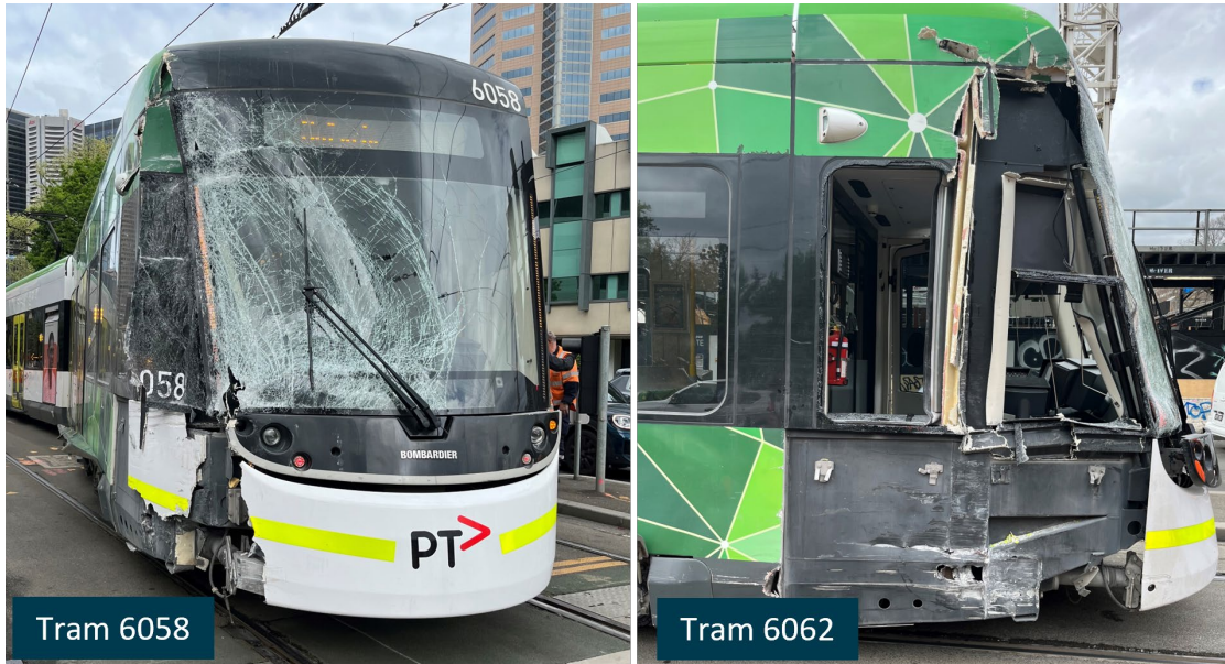
Figure 4: Damage to tram 6058 and tram 6062
